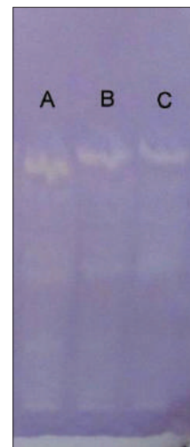
Figure 7: HPTLC-DPPH bioautography of PGGM samples exhibiting mild antioxidant activity. A = Mridu Paka, B = Madhyama Paka, C = Khara Paka
